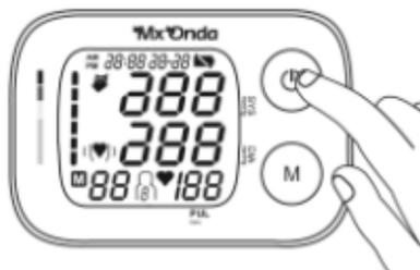
2. Once the wristband is inflated and the pulse is localized, the " ♥ " symbol will begin to flash at the pulse rate, the wristband will begin to deflate at constant speed and the display will show the value of the pressure decreasing
