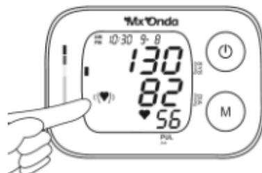
5. On the left side of the screen is the pressure indicator according to the classification criteria of the World Health Organization (WHO). This indicator consists of four marks or colors: green (normal tension), yellow (prehypertension), orange (high tension) and red (hypertension).
